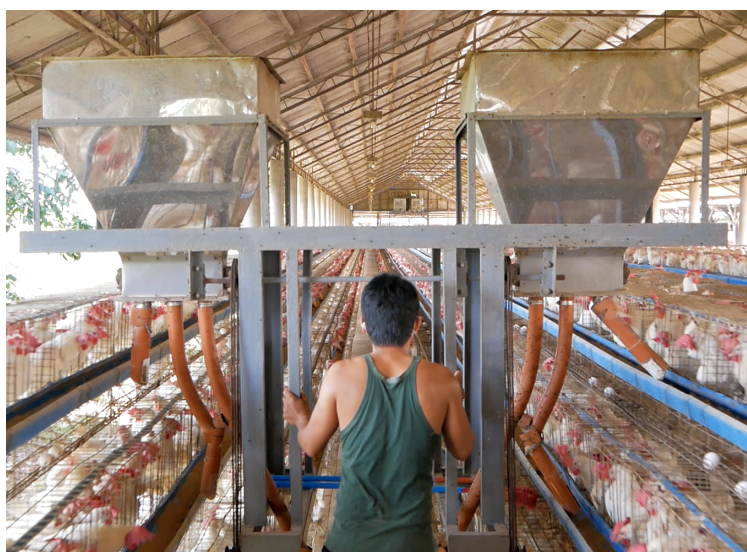
Ms. Cecille Aldueza Virtucio (top photo) and their farm worker (bottom photo) during the feeding of chickens in LMV farm, San Jose, Batangas. The farm worker is using their automated feeder system for chickens.
